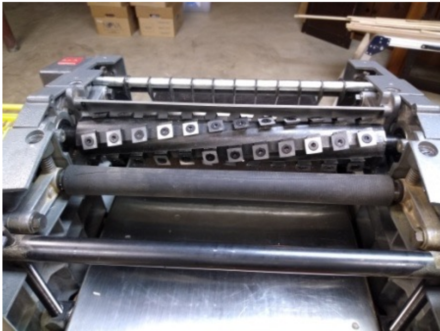
Cutter Head Installed in Planer
