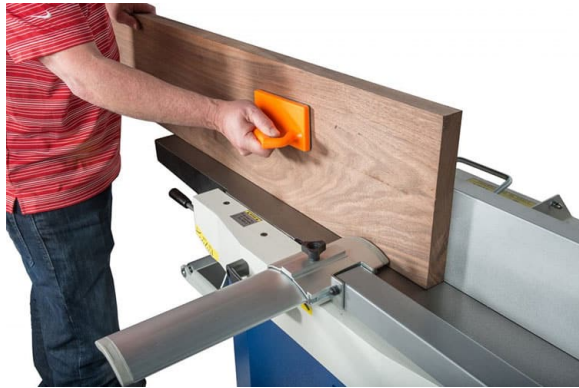
Squaring the edges on a jointer
